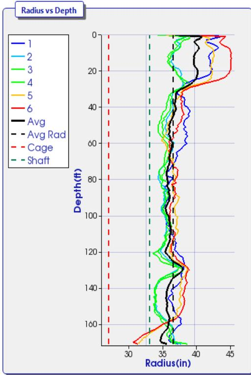
Estimated radius from temperature measurements of 1.68 m (5.5 ft) diameter shaft with 2.13 m (7 ft) diameter casing in upper 8.53 m (28 ft), I-90 bridge, Cleveland, Ohio. Shows that the as-built effective radius exceeds the design shaft radius ("Shaft") with adequate cover compared to cage location.
