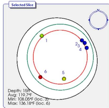
2-D slice of the upper 2.13 m (7 ft) diameter casing in upper 8.52 m (28 ft), I-90 bridge, Cleveland, Ohio. Slice shows a no offset of center of the casing from center of the main shaft.
