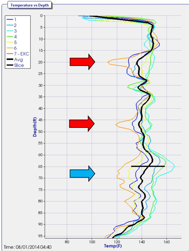
*Shaft with purpose-built defects (red arrows)*
