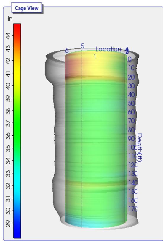
3-D rendering of 5.5 ft diameter shaft with 7 ft diameter casing in upper 28 ft, I-90 bridge, Cleveland
